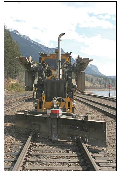
Nordco M7 Ballast Regulator/ Snow Fighter.
