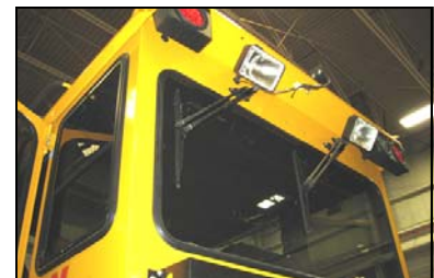
Window wiper arms installed on rear of TRIPP cab.
