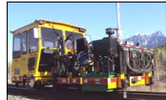
Nordco CX Hammer (top) and SP2R Dual Rail Spike Puller.
