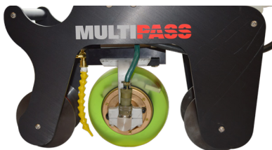
MultiPass inspection wheel includes six transducers for full rail inspection coverage.
