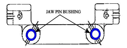
The steel bushing will wear longer than the bronze bushing in the 2135 8982 Jaw Mounting Assembly used on the Hydra-Hammer.
