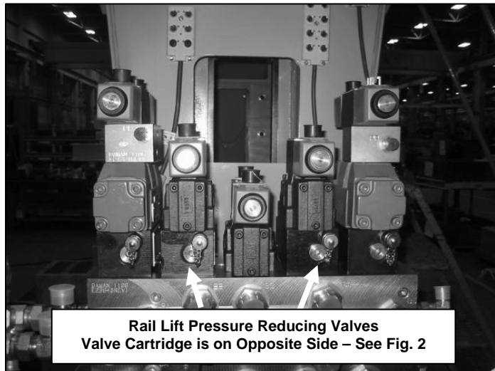
Figure 1 Rail Lift Manifold (Viewed from Front of Machine)
